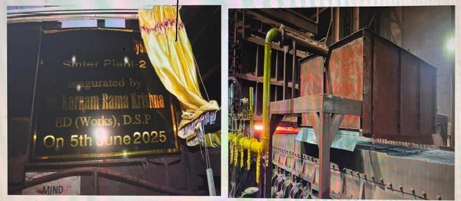
Under the decarburization initiative, Durgapur Steel Plant in collaboration with SAIL/RDCIS, successfully designed and implemented the system to **inject coke oven gas directly onto the sinter bed at Sinter Plant-2**. The system is envisaged to achieve a **reduction of approximately 3.5 kg of coke breeze per ton of gross sinter (TGS)**, translating to a net carbon dioxide **reduction of around 11 kg of CO2/TGS**.
