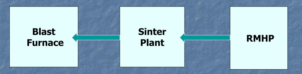
*To supply sinter to blast furnace of required \* Quantity \* Quality*
