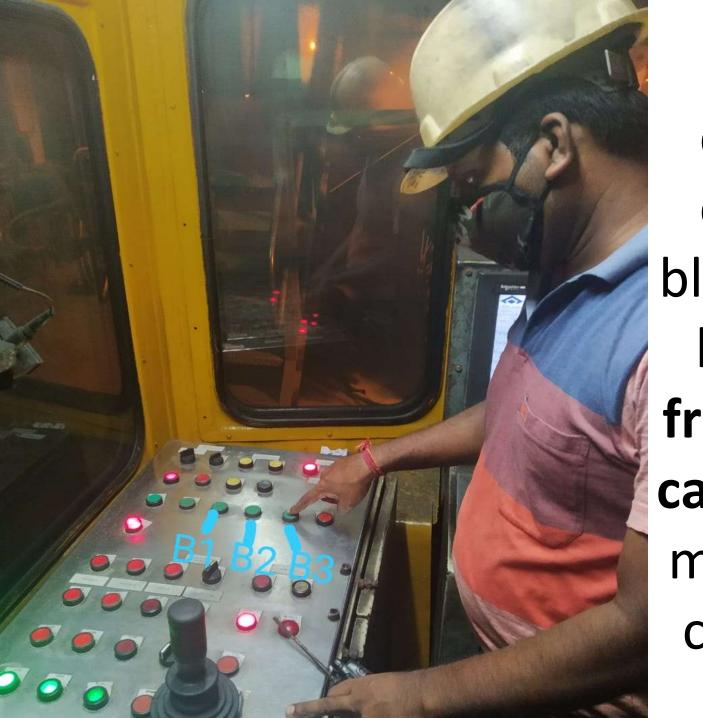
Both charging cars - air blasting can be done, from inside cabin, while monitoring coal level.
