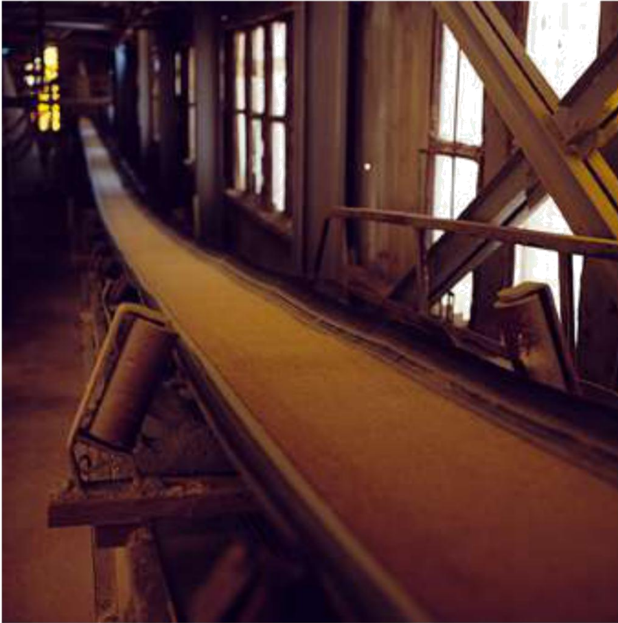
▲ Oily Fertilizer Belt 650 mm/EP 500
