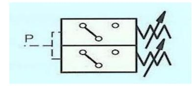
**LEVEL SWITCHES**: Generally the reservoir is provided with low level and high level float switches, so that they give alarm of low oil level/ high level and can be used for interlocking purpose. Float switch operates due to buoyancy in oil. Generally the low level
